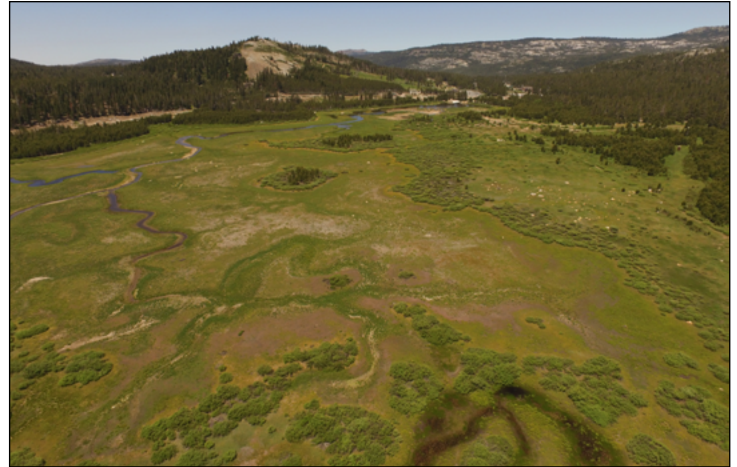
Downstream section of the meadow in relatively good condition. Little to no restoration actions planned in this area – no channel fill. This represents desired condition, with shallow, sinuous swales that has high floodplain connectivity and complexity. Credit: SYRCL drone footage.
