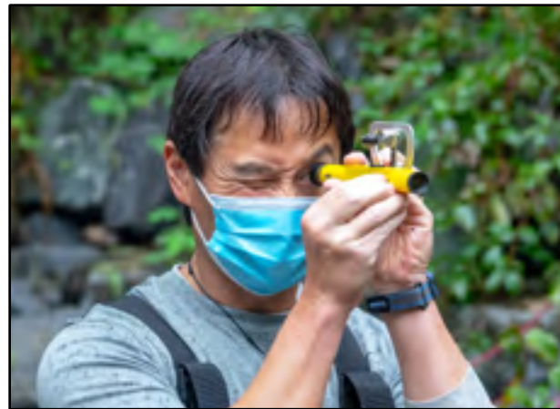
Dr. Dan McGarvey demonstrates using a clinometer to measure stream gradient.
